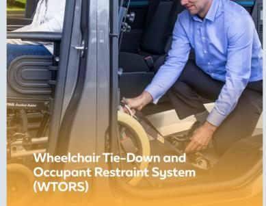
All Wheelchair Accessible Vehicles are fitted with some type of Wheelchair Tie-Down and Occupant Restraint System (WTORS). The purpose of WTORS is to provide safe restraint of both wheelchair and passenger during transport.
