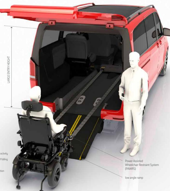
A lowered floor is not only better when travelling; the loading procedure is also made much easier for all. By lowering the floor, the gradient of the ramp is reduced.
