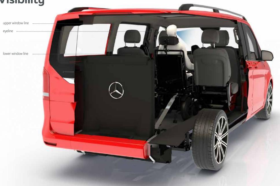
Ensuring that the wheelchair is positioned with all wheels on a level surface gives a much more natural seating angle, offering **improved visibility** out of the front and side windows.
